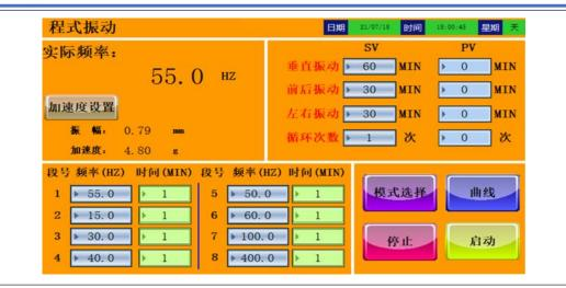
Octave sweep is continuous and its frequency should change with time according to the exponential law, sweep rate (sweep process of controllable variable frequency change rate of time df / dt) should be an octave per minute. There is a frequency range from  $f1 \rightarrow f2 \rightarrow f1$  sweep a test time (acceleration time), through the formula: 6.644log10 (high frequency / low frequency ) calculated from the results, and its sweep rate to ensure that the 1 octave / minute requirements.
